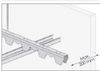
Where STEC 47/60 meets the wall, it is not necessary to have a perimeter profile.
